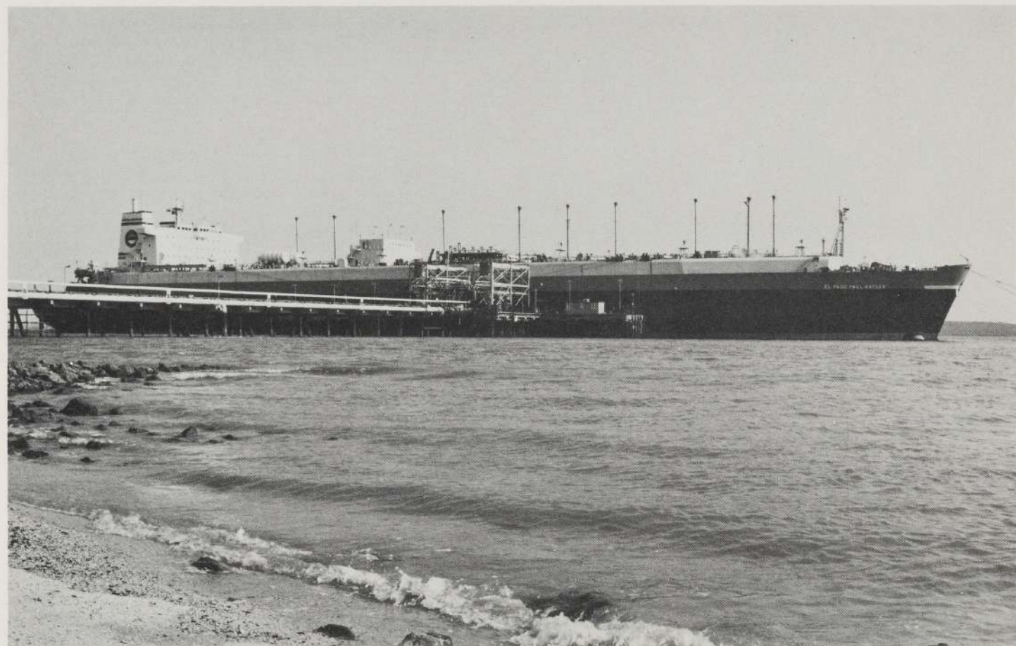
The LNG tanker, Paul Kayser , undergoing cryogenic tank cooling at the British Gas reception terminal at Canvey Island.
