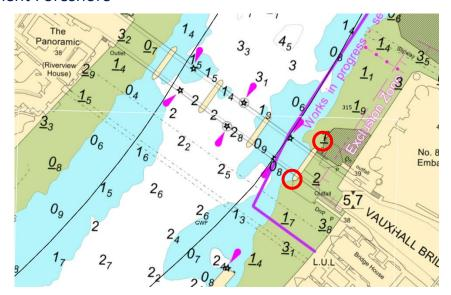
4.5. The lights will be mounted on masts at each site and will display two vertical yellow lights alternately flashing ½ second over a 1 second period. Albert site will also have a repeater light located on Vauxhall Bridge facing upriver between arches 4 &5, as shown on the chartlet above.
