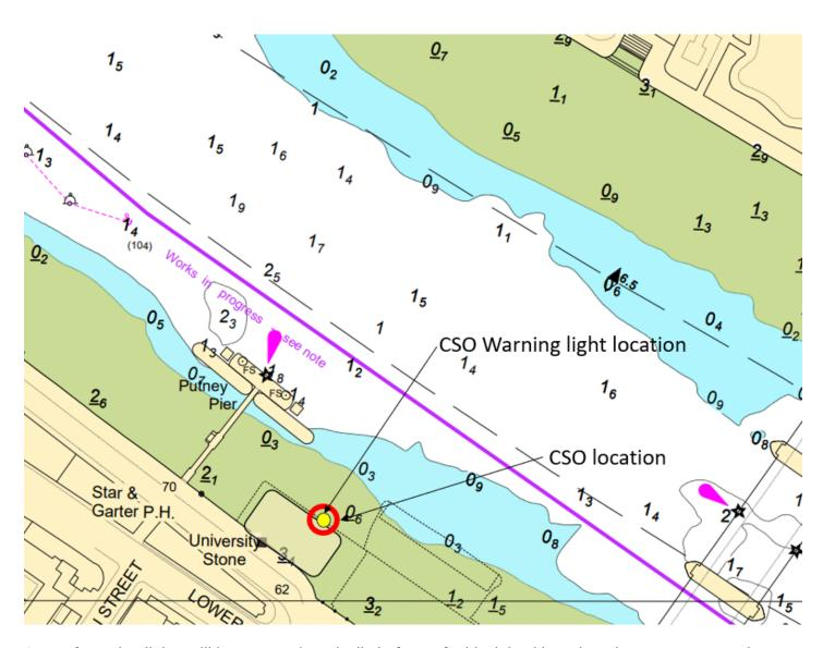
A set of warning lights will be mounted vertically in front of a black backboard on the permanent works structure embankment wall above the CSO with a set of repeater lights mounted above. The location of the CSO warning lights are marked in yellow on the above chartlet.
