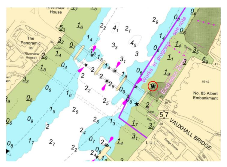
A set of warning lights are mounted vertically in front of a black backboard above the CSO and a repeater light is mounted on the upriver side of Vauxhall Bridge between arches 4 and 5. The location of the lights are shown on the chartlet (shown as black stars).
