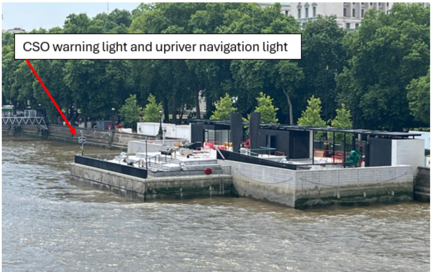
The lights will flash a yellow alternating 1 second pattern, visible day and night at a range of up to 200m, whenever the CSO is discharging or likely to discharge.
