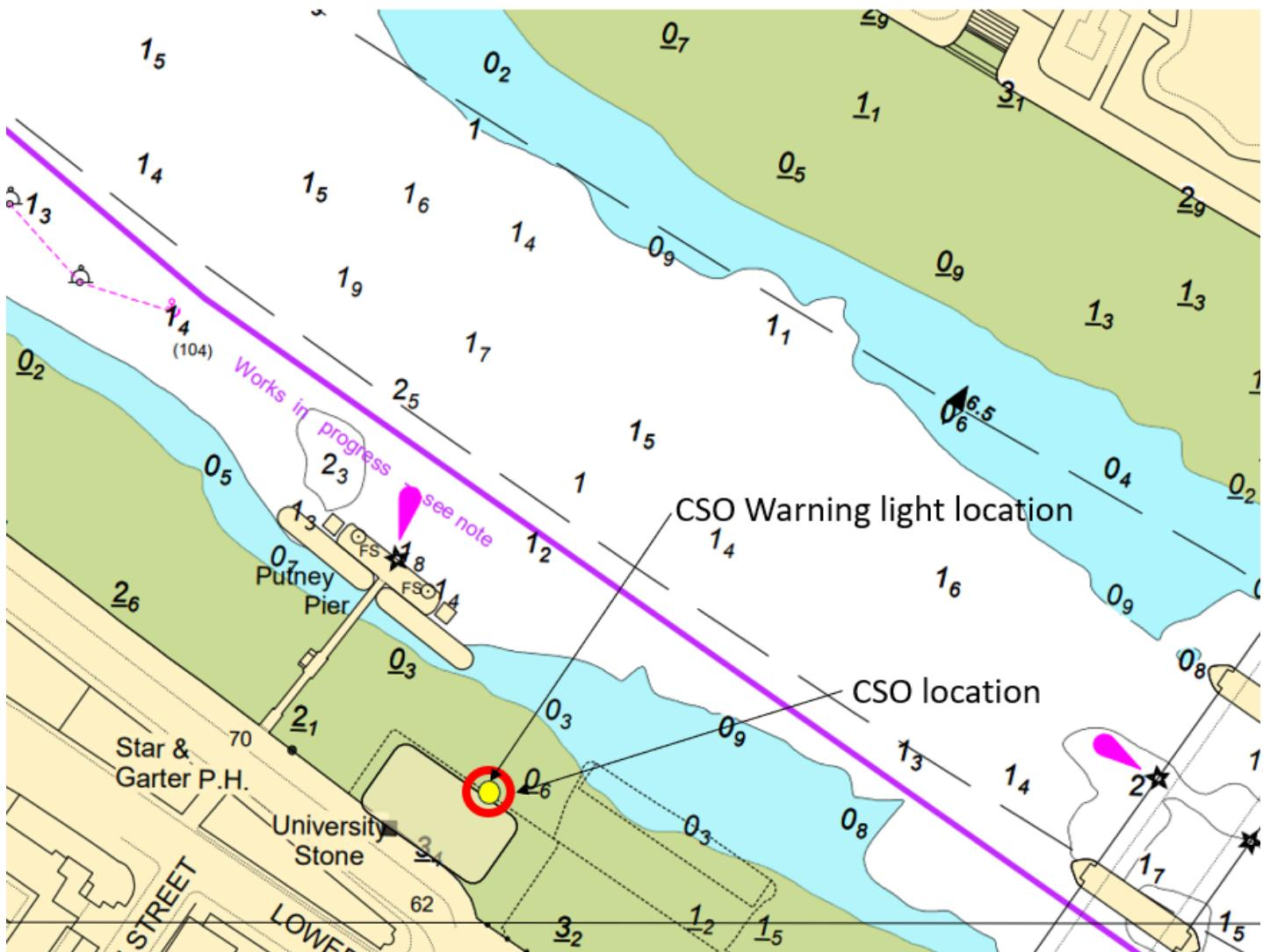
A set of warning lights will be mounted vertically in front of a black backboard on the permanent works structure embankment wall above the CSO with a set of repeater lights mounted above. The location of the CSO warning lights are marked in yellow on the above chartlet.
