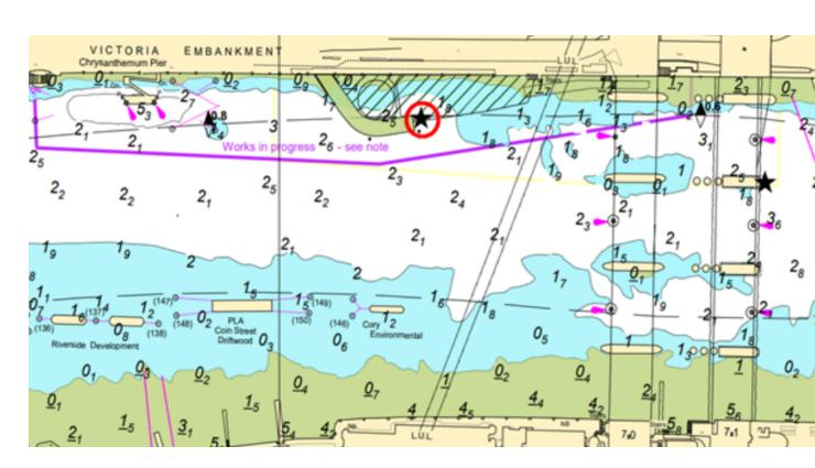
A set of warning lights will be mounted vertically in front of a black backboard on the riverwall above the CSO and a repeater light will be mounted above the bridge pier between arches 2 and 3. The locations of the lights are shown on the chartlet (shown as a black star).
