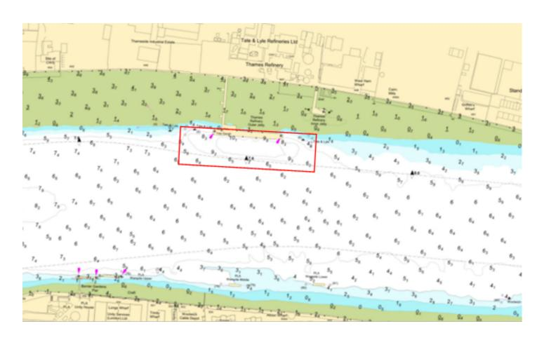
These dredging operations will be carried out by vessel **MAAS** or similar, using the water injection dredging method and will be conducted during ebb tides only.
