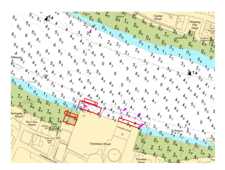
Works will involve the use of a JUB to the western end of the cofferdam which will extend beyond the LLAU (magenta line), a spudded barge to the front of the cofferdam and 1500t & 500t supply barges, which will occasionally be moored outside the LLAU but never overnight. Supply barges will be manoeuvred using the tugs SWS ENDURANCE, HANS and SUFFOLK.
