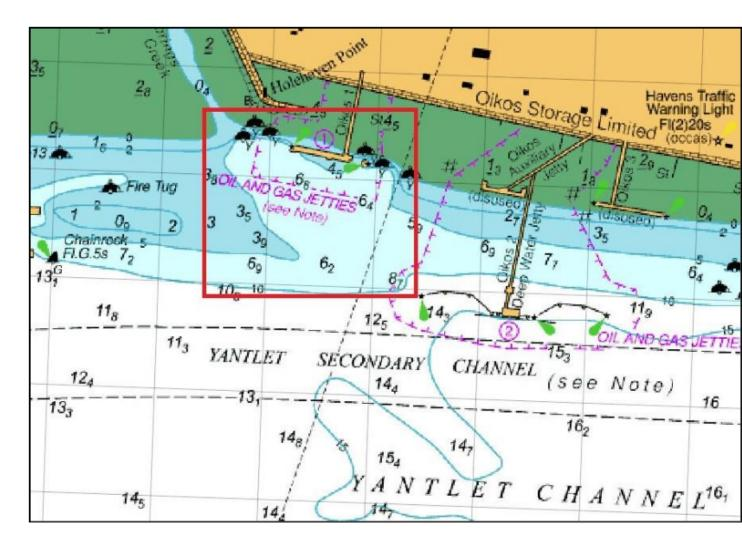
These dredging operations will be carried out by the Water Injection Dredging method and will be conducted during ebb tides only. The area to be dredged comprises the Oikos No. 1 Jetty berth box as well as the rear, clearance channel and the approach / transit area to the berth. The dredging is expected to be completed within approximately 12 days of commencement.
