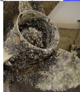
Boat Propeller covered in Quagga Mussel (© Utah Division of Wildlife Resources)
