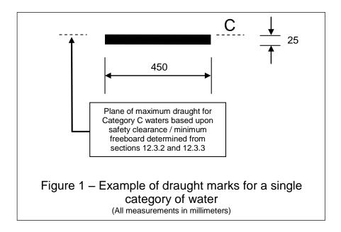
**12.3.6.** For vessels licensed to operate in more than one category of water, the draught marks referred to in Section 12.3.5 shall be supplemented by the addition of a 25mm wide vertical line to which one, or in the case of more categories, several lines shall be affixed. These affixed lines shall be positioned at the forward end of the basic marks and shall be 150mm long by 25mm wide. (See Figure 2).
