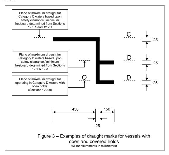
12.3.8. Vessels licensed to operate with both uncovered and weathertight holds bearing basic draught marks as required by Section 12.3.7 shall have the letter "O" marked at the after end of the basic draught marks relating to maximum authorised draught with uncovered holds. Such lettering shall be 60 mm high by 40mm wide. (Figure 3).
