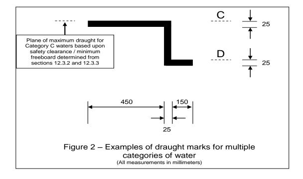
12.3.7. If the plane of maximum draught is determined by calculating that the vessel is weathertight when operating in Category D, and that the vessel meets only the minimum safety clearance of 750mm with covered holds (Section 12.1), then the maximum draught for operating with uncovered holds shall be determined and indicated by additional basic draught marks as prescribed in Sections 12.3.8 & 12.3.9.
