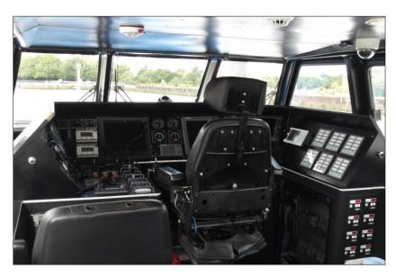
One incident highlighted the importance of a well laid out wheelhouse, as a Master reaching for poorly VHF Radio that was positioned contributed towards an incident. It is important to ensure that regularly used equipment, such as the VHF Radio, are within easy reach from the normal conning position, so that when used, the control of the vessel is not compromised.
