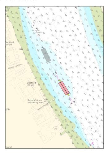
The barge mooring will be laid as a tier marked by unlit Admiralty class buoys at each end and identified as Deptford Strand Barge Moorings. It is anticipated this tier will be in place for the duration of the Tideway Tunnel workings.
