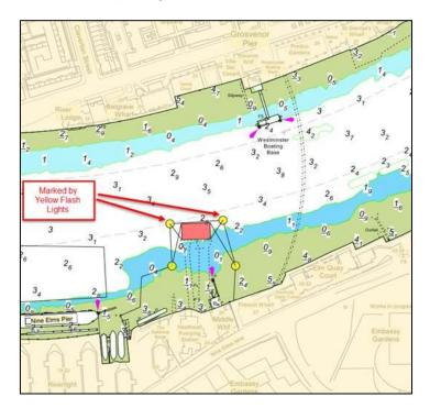
The works will involve the crane barge DEVON landing and lifting off a digger to and from the foreshore when accessible. The DEVON'S two anchor positons near the channel edge will be marked by yellow pellet buoys with flash yellow lights as indicated on the above chartlet.
