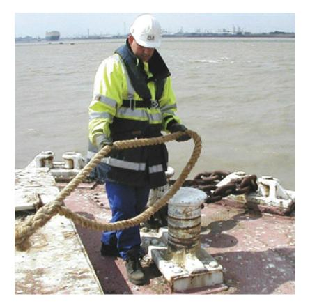
• Always hold a line by the side of the eye or the standing part. Throw the eye of a rope over a bollard or hook.
