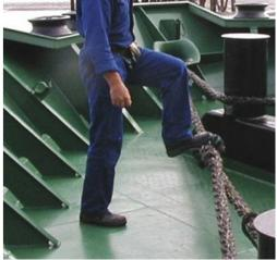
Walk over a slack mooring line between a bollard and a ship. Stand astride, stand on or walk over taut mooring lines. Stand
