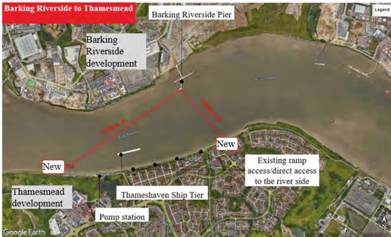
Figure 3: Crossing 3 – Barking Riverside to Thamesmead. The red squares indicatively show the proposed locations for the new pier (subject to detailed viability assessment and consent).
