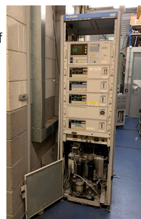
Figure 2 Horiba 9100 Mexa analyser at the laboratory of University College London
