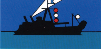
Vessel engaged in diving operations - by night
