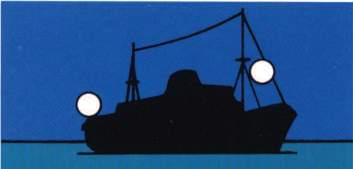
Vessel over 50 metres in length at anchor or moored
