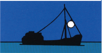
Vessel under 50 metres in length at anchor or moored
